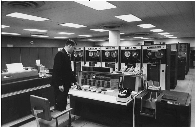
32K 36-bit words (147KB) memory, 0.5MHz clock, no disks (tape I/O)
